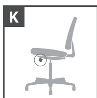
K. Tilt tension — Controls rate and ease of recline.
