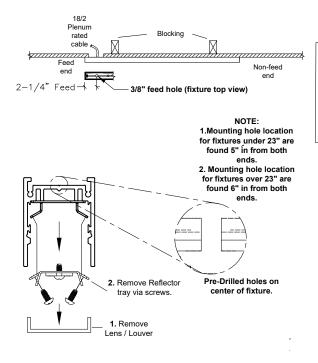
\*Note - Fixture mounting points are pre-drilled at 5" and 6" in from ends of fixtures. If alternate mounting points are req'd, drill & mount as necessary as shown on 1B.
