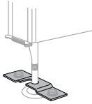
HAB Seismic Anchoring Bracket
