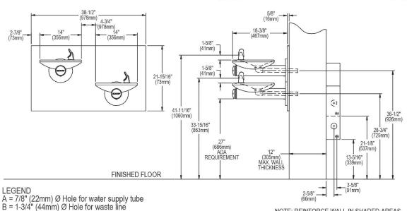
\*NOTE: ALL DIMENSIONS ARE TAKEN FROM THE FINISHED FLOOR ON THE SIDE OF THE WALL THAT THE FOUNAIN IS INSTALL ON.
