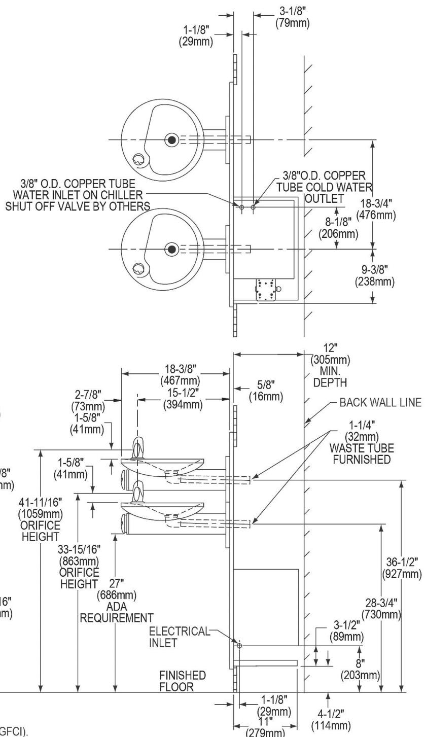
NOTE: New installations must use Ground Fault Circuit Interrupter (GFCI).
