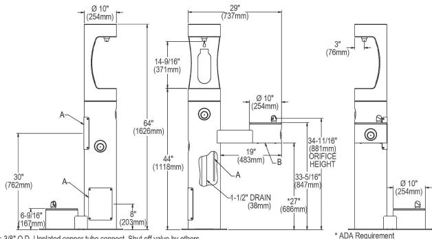
A = 3/8" O.D. Unplated copper tube connect. Shut off valve by others. B = Access panel (8" x 10").
