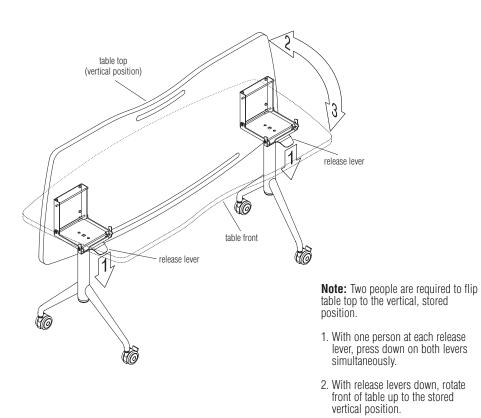
3. To return table top to the horizontal position, carefully rotate the top down and press down firmly until a "click" is heard at both flipping
