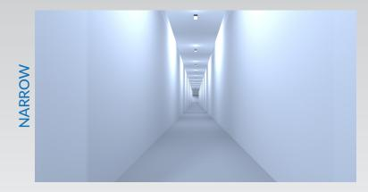
The narrow distribution optics align light along the length of the luminaire, allowing for superior vertical illumination in areas such as aisles or assembly zones.
