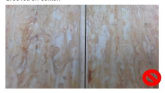
4. If the rod does not melt, it could be a symptom of a heat welding gun that is too cold or the operator is moving too quickly. The operator will need to decrease speed or increase temperature setting of the heath welding gun.
