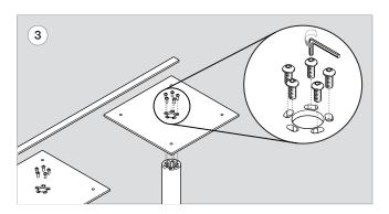
Flip the base. Using the 5/32" hex key, fasten the base to the mounting plates with 1/4 - 20 x 5/8" button head cap screw (x10). Align plates with a rule and tighten screws.
