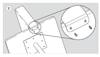
Using the 5/32" hex key, fasten the table divider with  $1/4 - 20 \times 5/8$ " button head cap screw (x4).
