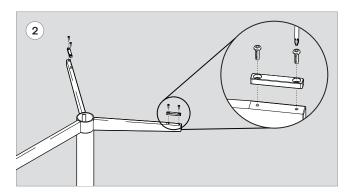
Using the Phillips screw driver, fasten each glide (x4) to the table base with #6-32 x 1/2" pan head machine screw (x8).
