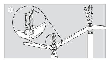
Using the 1/4" hex key, fasten each extrusion bottom to the table base with 1/4 - 20 x 1 3/4" socket head cap screw (x10) and 1/4" lock washer (x10).
