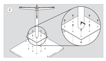
Using the 5/32" hex key, fasten the base sub assembly with 1/4 -  $20 \times 5/8$ " button head cap screw (x8).
