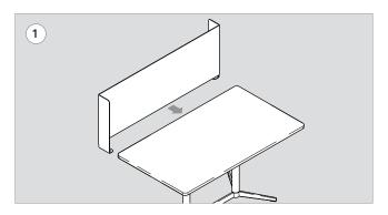
Slide table divider over the table top. Stop mid way to align the slots with the threaded inserts in the bottom of the table top.
