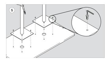
Flip the base. Using the 5/32" hex key, fasten the base sub assembly with 1/4 - 20 x 5/8" button head cap screw (x8).
