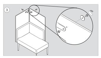
Using the 5/32" hex key, fasten bracket (x1) to divider (x2) with 1/4"-20 x 11/16" binder post and cap (x2), and 1/4" Flatwasher (x2).
