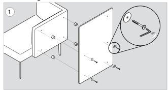
Using the 5/32" hex key, fasten divider to bench back with 1/4"-20 x 2 3/8" binder post (x4), spacer (x4) and 1/4" Flatwasher (x4).
