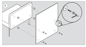
Using the 5/32" hex key, fasten divider to bench back with 1/4"-20 x 2 3/8" binder post (x4), spacer (x4) and 1/4" Flatwasher (x4).
