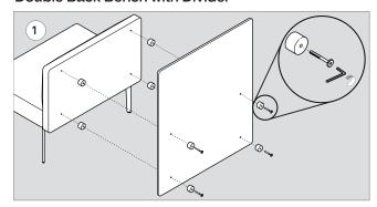
Using the 5/32" hex key, fasten divider to bench back with 1/4"-20 x 2 3/8" binder post (x4) and spacer (x8).
