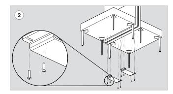
Using the 5/32" hex key, fasten ganging plate (x2) to bench (x2) with 1/4"-20 x 1" button head cap screw (x8)
