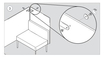
Using the 5/32" hex key, fasten bracket (x1) to divider (x2) with 1/4"- $20 \times 11/16$ " binder post and cap (x2), and 1/4" Flatwasher (x2).
