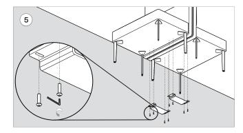
When ganging booths use the 5/32" hex key, fasten ganging plate (x2) to bench (x2) with 1/4"-20 x 1" button head cap screw (x8).
