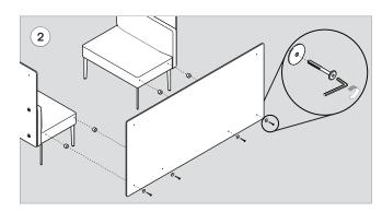
Repeat Step 1. Using the 5/32" hex key, fasten divider to bench seat side (x2) with 1/4"-20 x 2 3/8" binder post (x4), spacer (x4) and 1/4" Flatwasher (x4).
