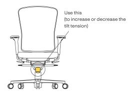
Use the big round knob undeneath the centre of the seat To increase tension turn the knob clockwise
