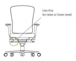
Use the paddle shaped lever on the right side underneath the seat To raise lift your weight off the seat while lifting the front of the lever To lower sit on the seat while lifting the front of the lever
