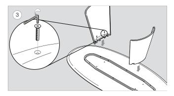
Install the table leg (x2) onto the table top and the steel frame at the four mount locations. Using the 5/32" hex key fasten with 1/4"- $20 \times 2$ " flat head cap screw (x8).
