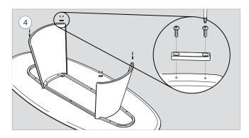
Using the Phillips head screw driver, install the glide (x4) using #6-32 x 3/4" rounded head screw (x8).
