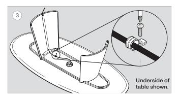
Using the Phillips head screw driver install the cable clamp (x1) with the #8-15 X 1/2" quad head wood screw.
