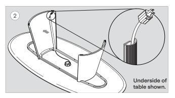
Remove the adhesive backing from the cable management track (x1) and press onto the center inside table leg. Feed the power cable into the cable management track.
