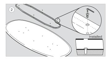
Using the 5/32" hex key, fasten the steel frame with 1/4"- $20 \times 5/8$ " button head cap screw (x6).
