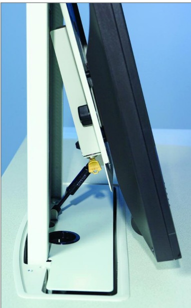
▲ A compact gas cylinder at the back of the monitor mount allows a tilt adjustment of 10° to minimize glare and create a preferred viewing angle. A locking device secures the LCD against tampering and theft.
