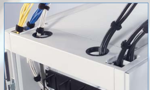
Separate, cable entry locations into the enclosure are provided for data and power. Reversible cable troughs allow secure cable routing from either the floor or the ceiling, or from a combination of both.
