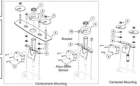
NOTICE! Sensor must be flush and parallel with the lens.
