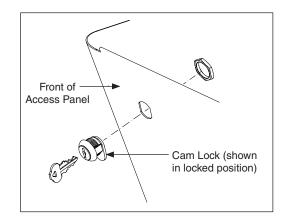
Position cam lock through access panel hole as shown and secure with nut (2 places).
