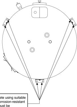
Secure the heater to the concrete using suitable concrete anchoring devices. Corrosion-resistant anchoring devices (8 places) must be 3" long x 3/8" diameter.
