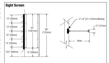
Generally recommended for sight screen application. Screen has floor mounting and requires minimum 3" concrete floor for anchoring.
