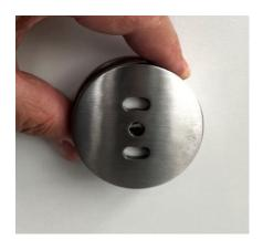
Place the retaining flange on the other side of the door over the latch opening. Thread the large screws into the back of the flange, and into the back of the knob on the other side of the door. Tighten the screws using a T-25 torx wrench.
