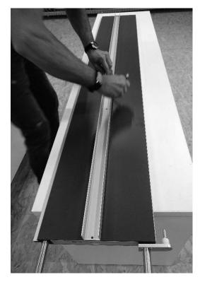
Using a 4.2 mm drill bit, drill the holes through the surface of the first panel only, and then attach the smaller U-bracket using 5.5 mm x 25 mm pan head
