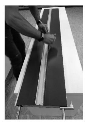
Using a 4.2 mm drill bit, drill the holes through the surface of the first panel only, and then attach the U-bracket using 5.5 mm x 25 mm pan head screws.
