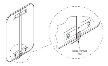
**Models 7B1-10XXXX and 7B1-30XXXX:** While holding the handle side of the mirror removal tool in one hand, insert the removal tool through the bottom center opening in the mirror shelf and then place the working end of the tool between the mirror and shelf.
