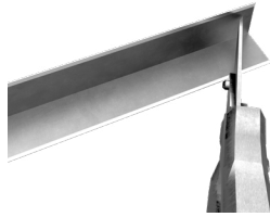
2. Miter adjacent molding
