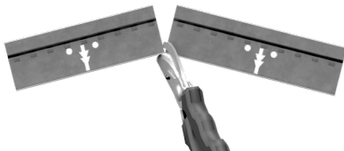
3. Bend and cut through flange of grid
