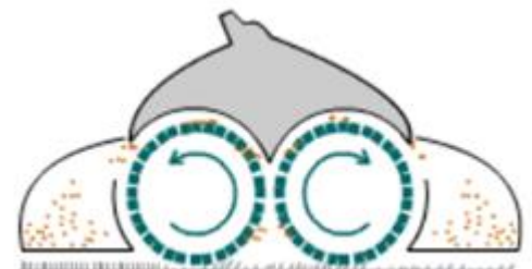
Twin Cylindrical Counter rotating brush machine cross section
