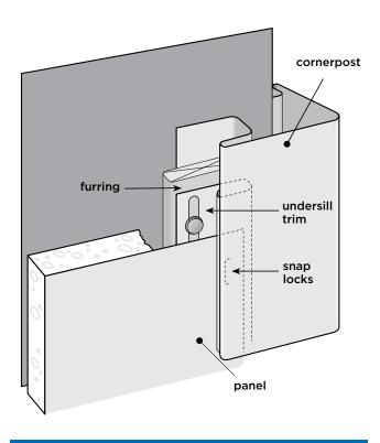
NOTE: When applying overlapping accessories, you may have to make new slots to avoid pinning the underlying accessory.
