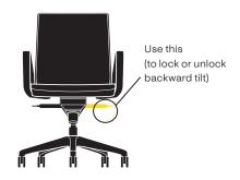
Use the paddle shaped lever on the left side underneath the seat. To unlock tilt pull the front of the lever up and tilt back slightly. To lock tilt recline to your desired position and push the front of the lever down.
