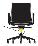
**Use** the big round knob underneath the center of the seat. **To increase** tension turn the knob clockwise.
