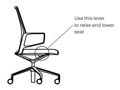
Use the lever on the right side underneath the seat
