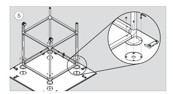
Using the 1/8" hex key, fasten the base sub assembly to the table top with with 10-24 x 1/2" flat head cap screw (x8).
