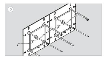
To link a power connection between multiple tables, the starter unit is energized, the connector units continue the daisy chain and the end unit completes the circuit.
