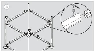
Install the side extrusion (x8) onto the eight top mount locations and the eight bottom mount locations. Using the 1/8" hex key fasten with 1/4"-20 x 5/8" set screw (x16).
