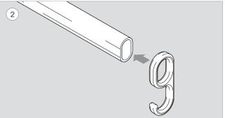
Slide the accessory hook (x2 or x4) onto the table side extrusion (x2 or x4).
