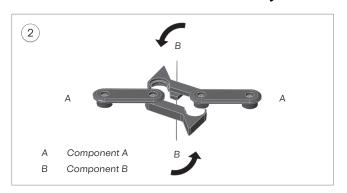
Rotate the Component B on each table until it clicks into Component A (See 1 & 2).
