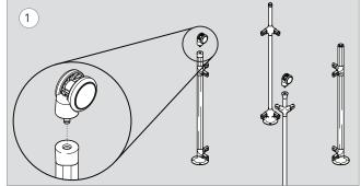
Place the glide leg sub assembly (x2) and caster leg sub assembly (x2) upside down as shown with legs with glides on one side and legs with casters on the other side. Press the caster (x2) into each caster leg bottom.
