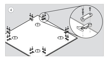
Place the table top upside down on a blanket. Using the Phillips head screw driver, install the ganging connector (x8) using 12-11 x 7/8" pan head wood screw (x16).
