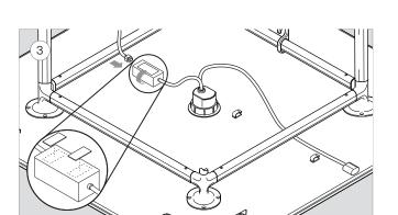
Place the cable management clip (x2) at the location shown. Fasten the control box to the underside of the table at the location shown using the provided velcro (x2)
