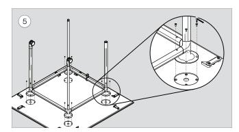
Using the 1/8" hex key, fasten the base sub assembly to the table top with with 10-24 x 1/2" flat head cap screw (x16).
