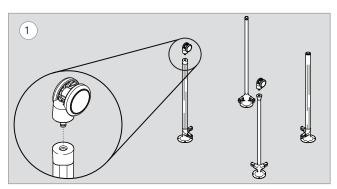
Place the glide leg sub assembly (x2) and caster leg sub assembly (x2) upside down as shown with legs with glides on one side and legs with casters on the other side. Press the caster (x2) into each caster leg bottom.
