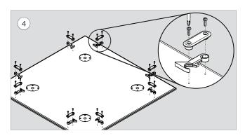
Place the table top upside down on a blanket. Using the Phillips head screw driver, install the ganging connector (x8) using 12-11 x 7/8" pan head wood screw (x16).
