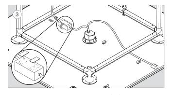
Place the cable management clip (x2) at the location shown. Fasten the control box to the underside of the table at the location shown using the provided velcro (x2)
