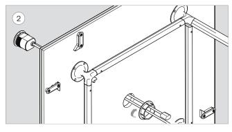
Unscrew the power box clamp and set aside. Feed the cable(s) through the table cut-out and power box clamp. Reinstall the power box clamp until hand tight.
