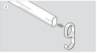
Slide the accessory hook (x2 or x4) onto the table side extrusion (x2 or x4).
