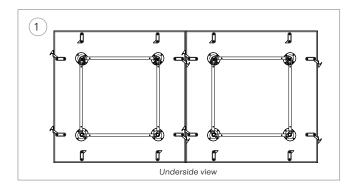
Rotate the Component B on each table until it clicks into Component A (See 1 & 2).
