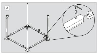
Install the side extrusion (x8) onto the eight top mount locations and the eight bottom mount locations. Using the 1/8" hex key fasten with 1/4"-20 x 5/8" set screw (x8).
