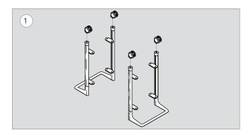
Place the handle sub assembly (x2) upside down on a blanket. Press the caster (x4) into each leg bottom.
