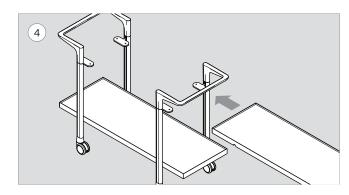
Turn the cart into the upright position. Slide the second shelf through the uprights in to the top position.
