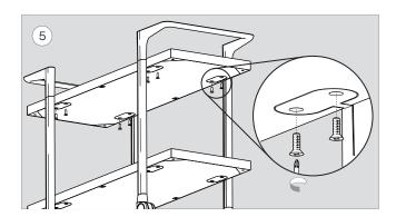
Using the Phillips head screw driver, fasten the second shelf with  $1/4-20 \times 3/4$ " flat head cap screw (x8).
