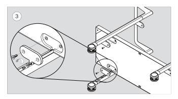
Lift the shelf on the opposite side. Slide the second handle sub assembly into position. Using the Phillips head screw driver, fasten with  $1/4-20 \times 3/4$ " flat head cap screw (x4).
