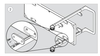
Using the Phillips head screw driver, fasten one handle sub assembly to a shelf with 1/4-20 x 3/4" flat head cap screw (x4) at the bottom mount locations.
