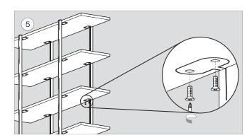
Using the Phillips head screw driver, fasten the remaining shelf platforms with  $1/4-20 \times 3/4$ " flat head cap screw (x24).
