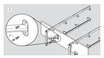
Using the Phillips head screw driver, fasten the two bottom supports using 1/4-20 x 3/4" flat head cap screw (x4).
