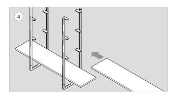
Turn the shelf into the upright position. Slide the remaining shelf platforms through the uprights in to position.
