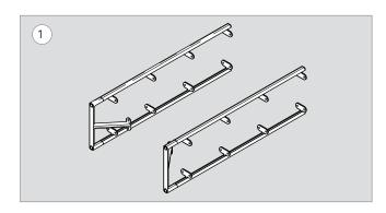
Place each column sub assembly (x2) on its side on a blanket approximately 28 inches apart.
