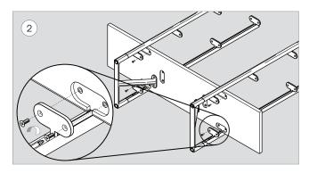
Using the Phillips head screw driver, fasten the column sub assembly (x2) to the bottom shelf platform with  $1/4-20 \times 3/4$ " flat head cap screw (x8).
