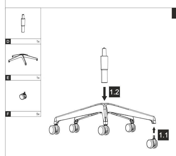
The pneumatic lift cannot be heated or dismantled. Replace it as a whole if necessary. The chair can be repaired or the chair components can be replaced only by trained staff.
