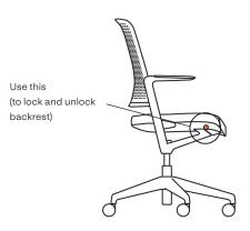
Use the button on the left and right side underneath the seat.
