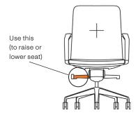
Use the paddle shaped lever on the left side underneath the seat To raise lift your weight off the seat while lifting the front of the lever To lower sit on the seat while lifting the front of the lever
