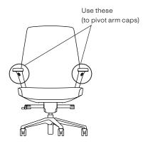
To rotate grasp the front of the arm rest firmly and pivot the arm cap inwards or outwards
