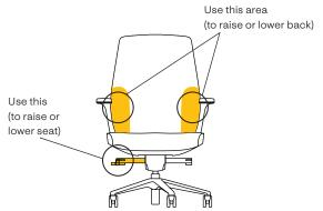
Use the paddle shaped lever on the right side underneath the seat To raise lift your weight off the seat while lifting the front of the lever To lower sit on the seat while lifting the front of the lever
