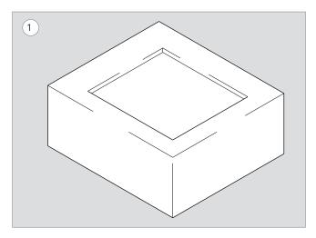
The platform base must be built with a window inset into the top surface that is 3/4" deep and have a mating surface within. The mating surface can be another panel or rails that stretch across the width of the window.
