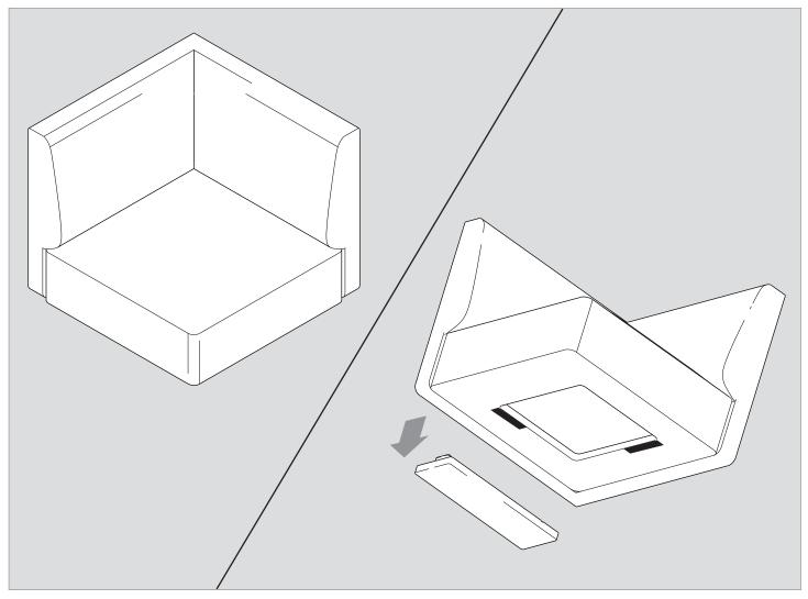
Each Pact Flex corner bench will come shipped on one mount. This mount is to be removed by pulling down at the rear to release the dual lock velcro. The mount will be installed into the platform base. The bench will have two pieces of dual lock velcro installed to accommodate the corner bench being installed to the left or right of an existing bench.
