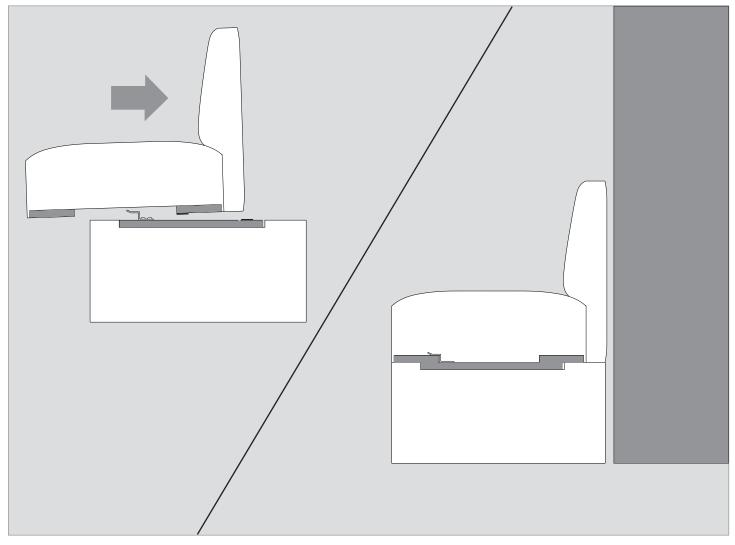
To install the Pact Flex bench, place the bench on the platform so the opening on the bottom panel sits over the attachment clips.
