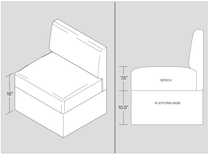
A standard Pact Flex bench has a seat thickness of 7.5 inches. In order to achieve an 18 inch seat height bench, a 10.5 inch platform base must be constructed. If a different seat height is required, adjust the height of the platform base. The installer is responsible for the remaining specifications of this platform base (i.e. weight capacity, finish and materials used).
