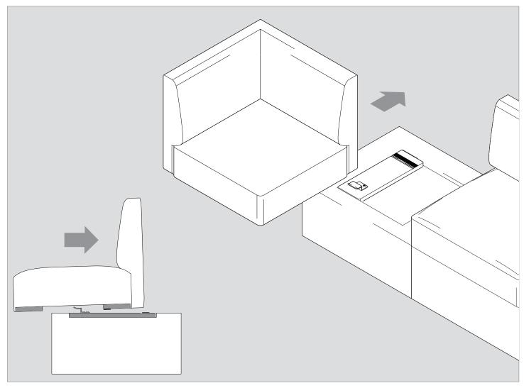
To install the Pact Flex corner bench, place the bench on the platform so the opening on the bottom panel sits over the attachment clip.
