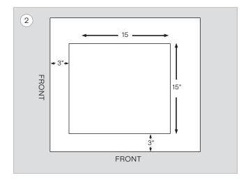
The width and depth of the inset window is 15 inches. For the Pact Flex corner model to finish flush with the front surface of the platform, the window must be inset 3 inches from the front edge. Two fronts are shown as the corner unit can be installed to the left or right of an existing bench.
