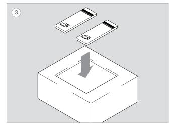
Using #10 wood screws that are at least 11/2" long, install the Pact Flex mounts to the mating surface within the top platform window. Screws are not supplied by Keilhauer.
