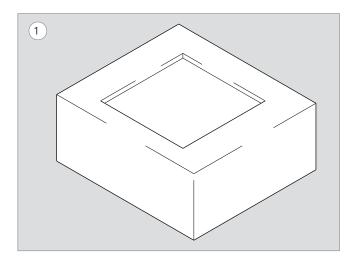
The platform base must be built with a window inset the top surface that is 3/4" deep and have a mating surface within. The mating surface can be another panel or rails that stretch across the width of the window.
