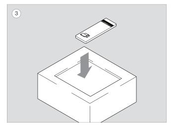
Using #10 wood screws that are at least 11/2" long, install the Pact Flex mount to the mating surface within the top platform window. Screws are not supplied by Keilhauer.
