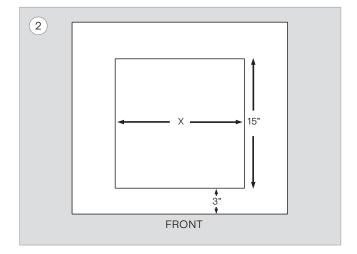
The centered width of the inset window (x) is 10 inches less the width of the Pact Flex model. The depth is 15 inches. For the Pact Flex model to finish flush with the front surface of the platform, the window must be inset 3 inches from the front edge.
