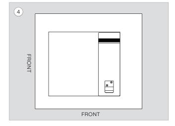
The Pact Flex mounts must be flush with the side of the inset window to allow the dual lock velcro to align with the bench. Two fronts are shown as the corner unit can be installed to the left or right of an existing bench.
