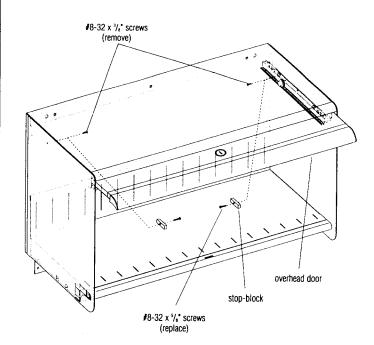
**Note:** The instructions below are to install a stop-block into the mechanism of the cabinet. The block is used to stop the overhead door from receding fully when the key is left in the door.
