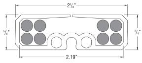
Note: 1/4" dia. cables shown in cavity as reference.
