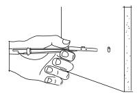
2.2) Hold ends of strap between thumb and forefinger and pull toward you until channel rests flush behind wall. While holding the strap/channel in place, slide the plastic cap along the straps until the flange of the cap is flush with the wall.
