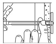
2.3) Snap the plastic straps off by pushing from side to side. Ensure the straps are level with the cap.
