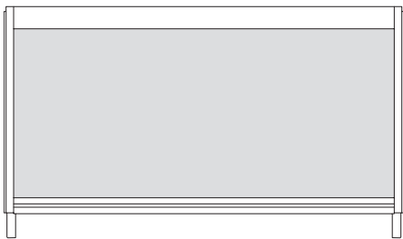
Framed glass with integrated mounting rail
