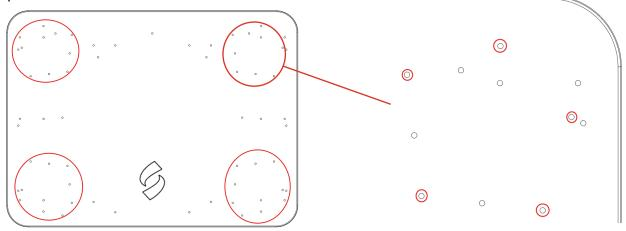
**Step 2:** Align table leg with pattern and install the corresponding screws. **Make sure to only use plastite screws on hard plastic tops and wood screws on wood tops.** Repeat for each leg.
