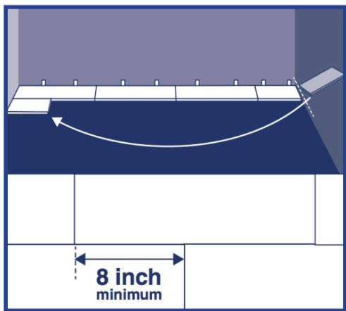
Step 3: Use leftover plank from first row as starter for second row. There must be at least 20cm (8in) between plank end joints on adjacent rows.
