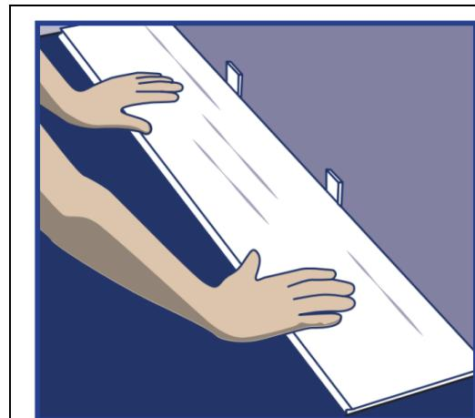
Step 1: Begin installation working from left to right. Insert spacers at ends and edges where planks meet wall.
