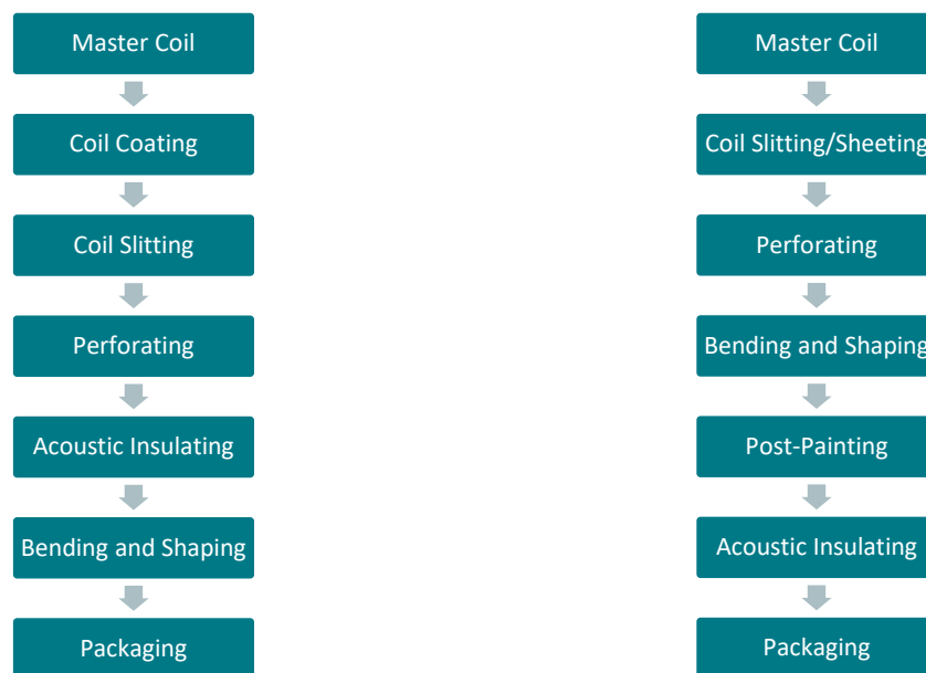
Figure 1: Typical aluminum specialty product manufacturing process, coil-coating (left) & post-painting (right)
