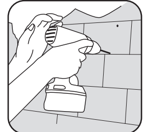
4. Drill holes. Drill holes for screw anchors.
