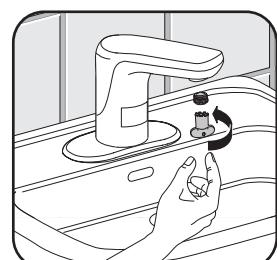
6. Install outlet and tighten with outlet key (supplied).
