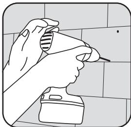
2. Drill holes for screw anchors.
