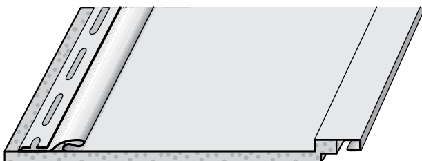
Single 12" Vertical Board and Batten
