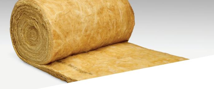
High Temperature Blanket is composed of rotary glass fibers bonded together using a thermosetting resin and formed into plain, flexible and resilient thermal insulation. It is designed for use on industrial equipment, panel systems, pipe fittings and tanks operating at temperatures up to 1000°F (538°C). Type I is available in either batt or roll form; Type II is available only as batts. HT blankets are easy to handle, cut with a knife and install, and contain over 60% recycled glass content.
