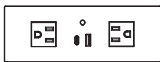
PX2 6 5 / 8 " W x 2 1 / 2 " D Two outlets, one USB-A and one USB-C charging port
