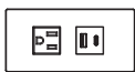
PX1 5 1 / 4 " W x 2 1 / 2 " D One outlet, one USB-A and one USB-C charging port
